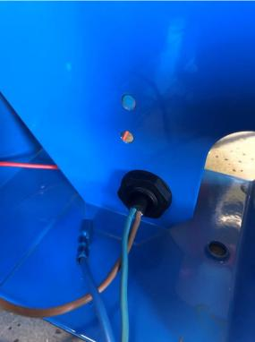
11. Connect and install the starting compressor (observe correct polarity! Red cable is +):
