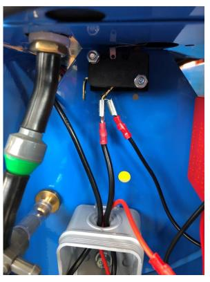
17. Lead the red cable coming from the battery tube through the distribution box and connect it to the micro switch:
