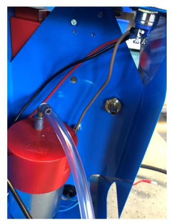
15. Lead the black cable coming from the start button through the distribution box and connect it to the micro switch:
