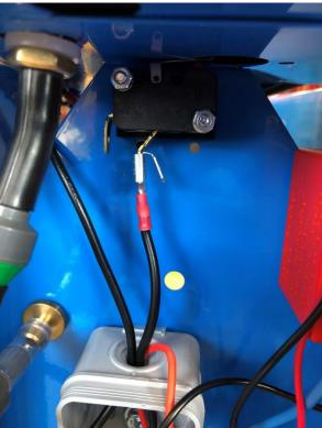
16. Connect the black cable coming from the ignition coil to the micro switch:
